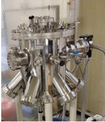
図3 CoCrFeMnNi-HEA 用スパッタ装置. The figure is taken from Applied Physics Letters, vol. 124 (2024) 151903.
