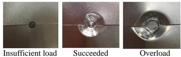
Fig. 4 Appearances of welded specimen
