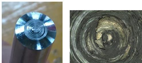
Fig. 6 Adhesion of workpiece to tool surface.
