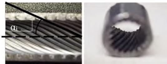
Fig.4 Example extruded circular tube with many spiral projections on inside wall
