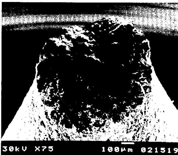
Fig.5 SEM photographs of the fracture surface of the \beta -spodumene glass-ceramics (Deformation temp.:1470K)
