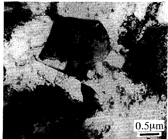
Fig. 5 Transmission electron micrograph of the laminations of Mg-5Al-1Y alloy after consolidation by a hot upsetting at 573K.
