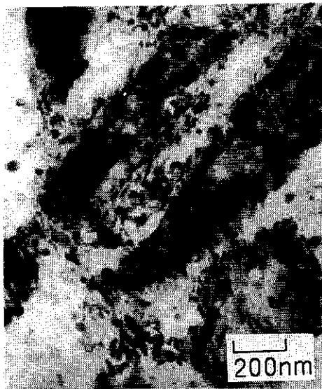
Fig. 2 Transmission electron micrograph showing a microstructure of ribbon at a plane parallel to the chilled surface of Mg-5Al-1Y alloy.
