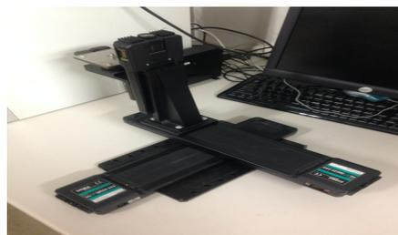
Fig. 2 A view of X-Y stage for laser irradiation.
