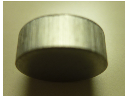
Fig. 18 Photograph of cut surface of fine-blanking for SPCC
