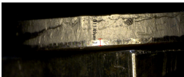
Fig.10 Sheared surface of S45C (Maximum)
