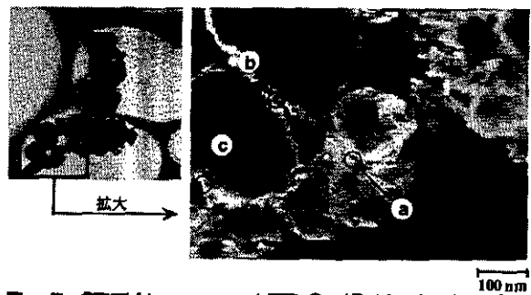
Fig. 7. STEM image and EELS (B-K edge) of ceramics (SiC+BN) for a, b, c, areas and h-BN as standard.
