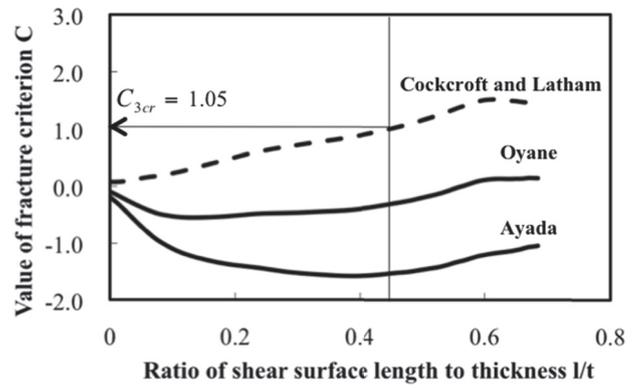
Fig.14 Relationship between sheared surface length and value of each fracture criterion (SPCC)
