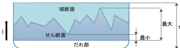
Fig.6 Schematic figure of cut surface for experiments
