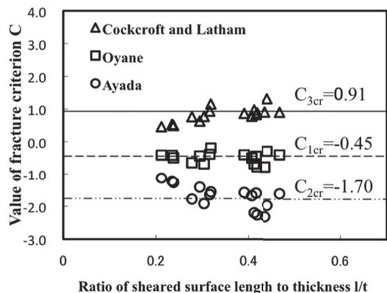
Fig.16 Relationship between sheared surface length and value of each fracture criterion (SPCC)
