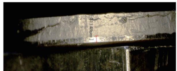
Fig.10 Sheared surface of S45C (Maximum)
