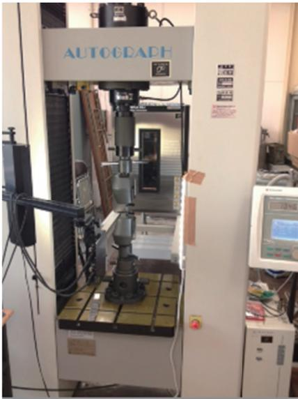
Fig.2 Universal tensile and compression testing machine
