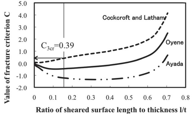
Fig.15 Relationship between sheared surface length and value of each fracture criterion (S45C)
