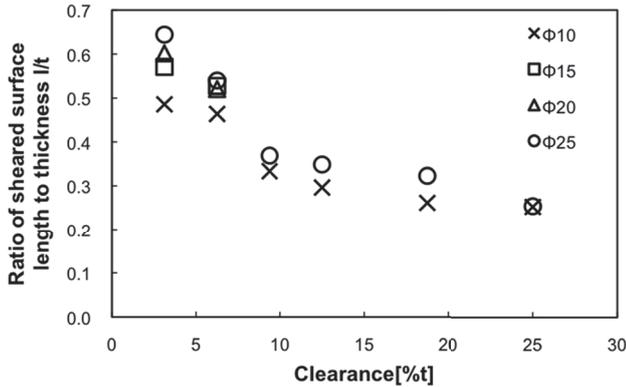
Fig.12 Relationship between clearance and sheared surface length (SPCC)
