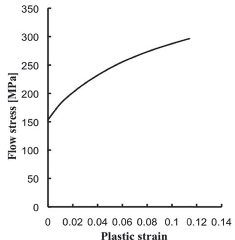
Fig.4 Flow stress-plastic strain relation for SPCC
