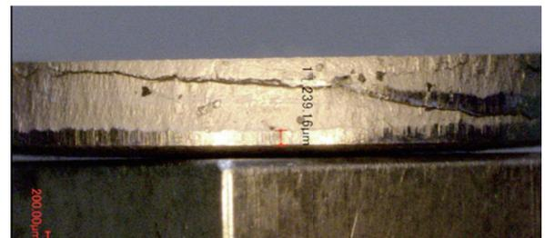
Fig.9 Sheared surface of S45C (Minimum)
