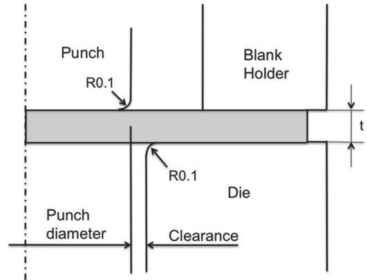
Fig. 3 Axisymmetric model for analysis
