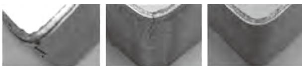
▲ Crack+peeled of Al    △ Crack    ○ Formable
