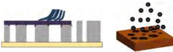
Fig.20 Schematic illustration of the lotus copper plates surface to the wire blush and shot peening surface
