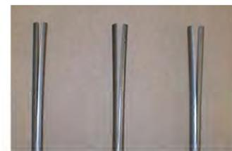
**Fig. 7** Experimental results of slit method of bar drawn with type dies
