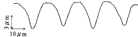
Fig.11 Example of dimple profile
